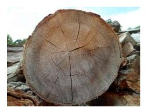
Short clip – Glenn Lucas processing a log... eliminate the pith, create platters or plates from the quarter sawn sections on either side of the pit, use a sharp chain in order to cut straight.
